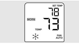
Figure 7: Temperature Setpoint Example
